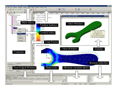
The **View Window** shows the model itself. Each view window is completely independent and may show the model from a different angle, using different visualization options, with or without results. The image in a view window is built up from several drawing layers as listed in the layers panel in the Tree Frame. Each draws over the top of the one before it. In the example shown, Window 2 draws geometry first, then contours, then mesh, then annotation.
